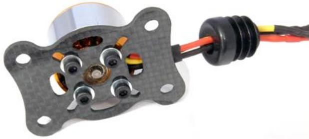
**NOW IT'S TIME FOR MOUNTING YOUR 6 MOTORS. USE THE M3 X 6 ALLEN CAP BOLTS, AND THE M3 WASHERS. USE AS WELL SOME LOCKTITE.**
