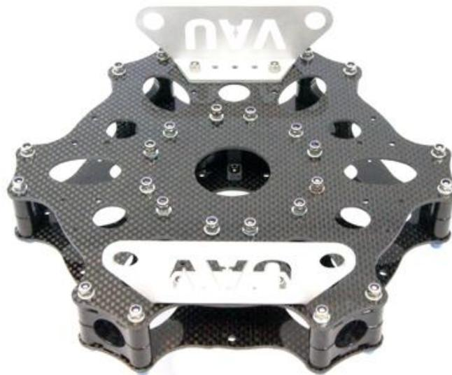
**ALL BOLTS AND LOCKNUTS ARE STILL ONLY HAND TIGHTENED**
