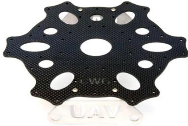
**MOUNT THE ALUMINUM BRACKETS/ WIREDAMPERSYSTEM (IF BOUGHT SEPARATELY) TO THE BOTTOM CENTERPLATE, YOU CAN LET THE LOGO POINT UP OR DOWNWARDS, CHOOSE HERE TO FLY IN + OR X MODE, THE HOLES ARE FOR BOTH MODES ALREADY PRE- DRILLED AS WELL FOR BIGGER AND SMALLER LANDING GEARS**
