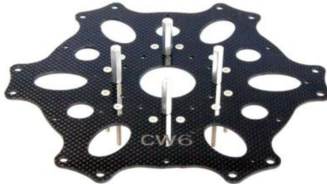
**TAKE THE UPPER CENTERPLATE (YOU CAN RECOGNIZE THIS PLATE WITH THE COUNTERSUNK HOLES). LET THE LOGO (CW6) POINT UPWARDS.**
