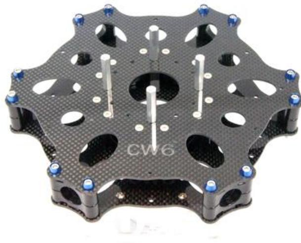
**NOW YOU CAN TAKE THE ALLEN CAP BOLTS M3 X 35 AND THE ALUMINUM CAPS, 6 PAIRS OF BOOMCLAMPS, 12 LOCKNUTS AND 12 M3 WASHERS MOUNT THEM AS PICTURE ABOVE AND BELOW**
