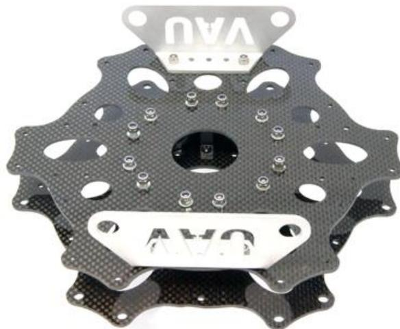
**AT THIS POINT YOU PUT THE LOWER CENTERPLATE (LOGO'S ALIGNED) OVER THE COUNTERSUNK BOLTS . YOU CAN MOUNT THE WASHERS AND THE LOCK NUTS ON THE 12 COUNTERSUNK BOLTS, JUST TIGHTEN THEM A FEW TURNS, SO THEY WILL NOT COME OFF.**
