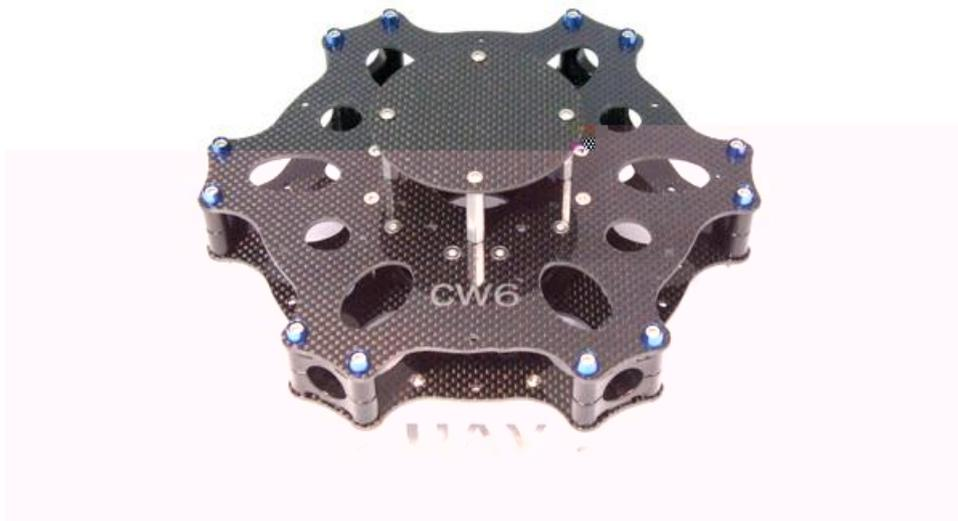
**ON THE PICTURE IS THE "MOUNTING PLATE SMALL" SHOWN, MAKE SURE YOU POSITION IT FOR + OR X MODE (PICTURE IS X MODE)**
