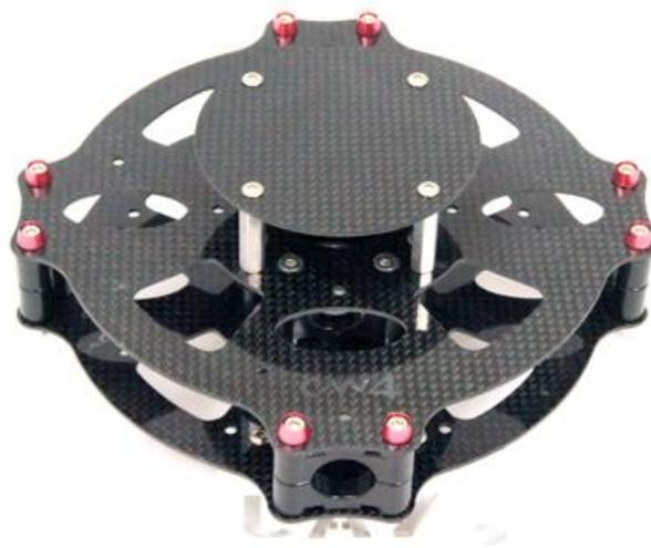
**ON THE PICTURE IS THE "MOUNTING PLATE SMALL" SHOWN, MAKE SURE YOU POSITION IT FOR + OR X MODE (PICTURE IS X MODE)**
