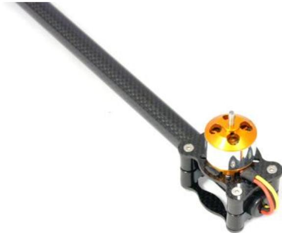
**NOW YOU CAN MOUNT THE MOTOR PLATES TO THE TUBE, AND PUT THE ENDCAP IN THE TUBE, JUST LIKE ON THE PICTURE, MAKE SURE YOUR CABLES ARE CONNECTED INSIDE THE TUBES CORRECTLY OR MAKE SURE THE CABLES ARE LONG ENOUGH TO REACH YOUR ESC. AT THIS POINT YOU CAN TIGHTEN THE BOLTS. DO NOT OVERTIGHTEN THE CLAMPS CAN BREAK WHEN YOU OVERTIGHTEN THEM A LOT. MAKE SURE THE CLAMPS ARE CLOSED TO EACHOTHER LEFT AND RIGHT THE SAME.**
