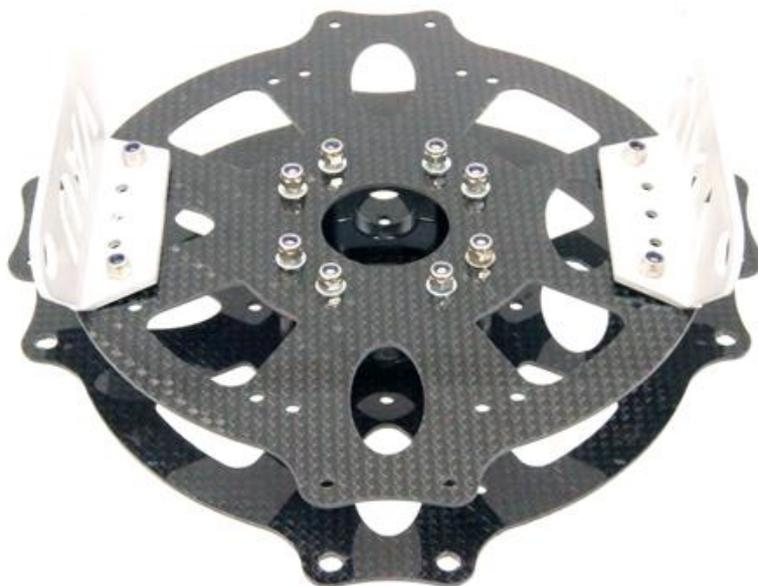
**AT THIS POINT YOU PUT THE LOWER CENTERPLATE OVER THE COUNTERSUNK BOLTS .MAKE SURE THE LOGO'S OF BOTH PLATES ARE ABOVE EACHOTHER (ALIGNED) YOU CAN MOUNT THE WASHERS AND THE LOCK NUTS ON THE 8 COUNTERSUNK BOLTS, JUST TIGHTEN THEM A FEW TURNS, SO THEY WILL NOT COME OFF.**
