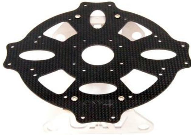
**MOUNT THE ALUMINUM BRACKETS/ WIREDAMPERSYSTEM (IF BOUGHT SEPARATELY) TO THE BOTTOM CENTERPLATE, YOU CAN LET THE LOGO "CW4" POINT UP OR DOWNWARDS, CHOOSE HERE TO FLY IN + OR X MODE, THE HOLES ARE FOR BOTH MODES ALREADY PRE- DRILLED AS WELL FOR BIGGER AND SMALLER LANDING GEARS**
