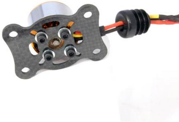
**NOW IT'S TIME FOR MOUNTING YOUR 4 MOTORS. USE THE M3 X 6 ALLEN CAP BOLTS, AND THE M3 WASHERS. USE AS WELL SOME LOCKTITE.**
