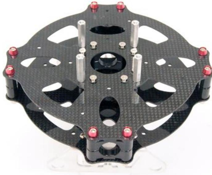
**NOW YOU CAN TAKE THE ALLEN CAP BOLTS M3 X 35 AND THE ALUMINUM CAPS, 4 PAIRS OF BOOMCLAMPS, 8 LOCKNUTS AND 8 M3 WASHERS MOUNT THEM AS PICTURE ABOVE AND BELOW**
