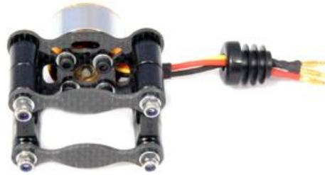
**USE FOR EACH MOTOR PLATE 2 PAIRS OF CLAMPS, 4 M3 WASHERS, 2 MOTORPLATE POSITION PLATES, 4 M3 X 35 BOLTS AND 4 M3 LOCKNUTS, JUST TIGHTEN THEM WITH YOUR HANDS**
