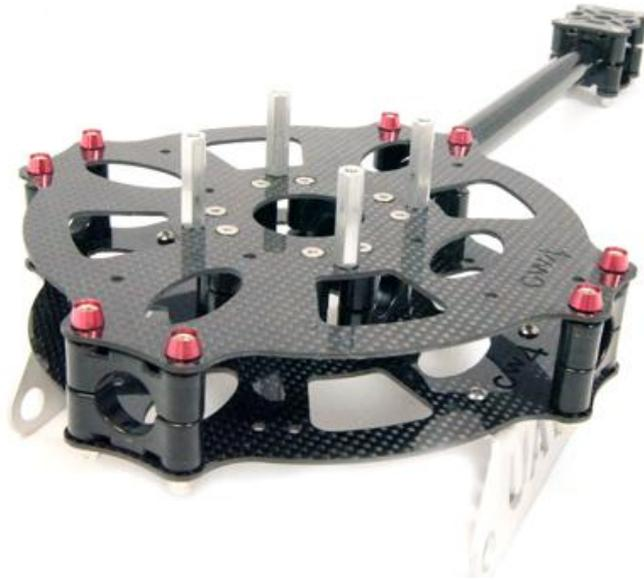
**NOW YOU PUT ALL ARMS INTO THE CENTERUNIT. AND LOCK THE BOLTS AND NUTS. MAKE SURE ALL MOTORS ARE LEVELED CORRECTLY IN LINE OF THE CENTERUNIT.**
